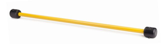
Integrated target holders on each end are positioned off-axis and allow the SMR to rotate 360° for easy visibility. A new 3-point mount constrains the bar in the field exactly as it is certified at the factory to assure the highest accuracy possible.
