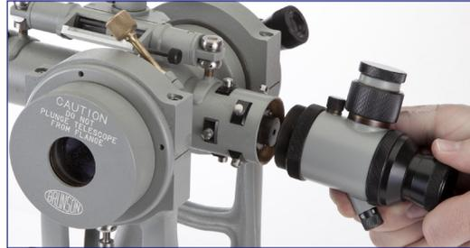
8440 AlignCam eyepiece removal.
