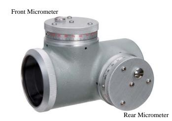
Initially set the rear micrometer to zero in preparation for calibrating the front micrometer.
