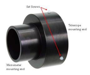
When securing the adapter to the telescope barrel, do not over tighten the set screws as barrel distortion may occur.
