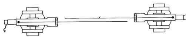
A. BOTH INSTRUMENTS FOCUSED ON INFINITY PARALLEL BUT NOT COINCIDENT.
