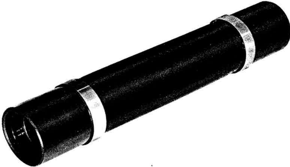
Fig. 114. K&E Collimator 9092-30 for checking straightness of line of sight.
