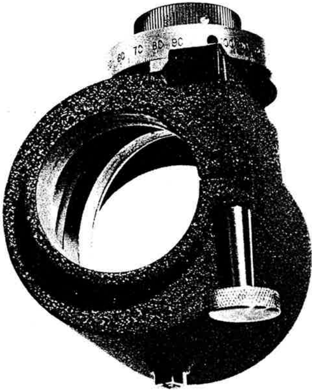
Fig. 40. The Optical Micrometer. The instrument is shown as it would appear from the direction of the operator when installed on a Jig Transit. The lower right hand screw clamps the instrument in position. The upper knob and drum control the planoparallel plate. The plate is shown tilted sideways so that it would move the line of sight 0.081 inch to the right, as shown by the reading on the drum.
