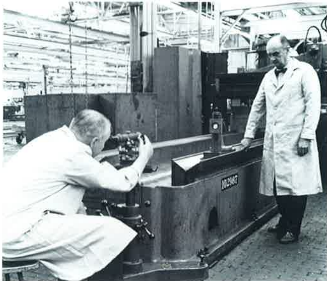
K&E Tilting Level checks ways of 30-foot horizontal milling machine for both twist and sag within .002 inches
