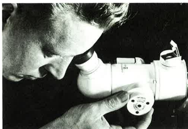
With optical telescopes, line of sight replaced the traditional piano wire methods, to erect and position huge jigs, fixtures and machinery.
