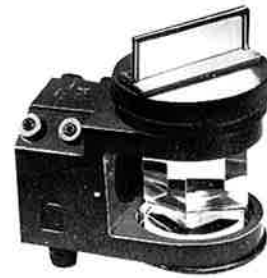
Figure 3-14. The plating prism. When the prism is rotated, the line of sight sweeps a plane. By rotating the telescope, the slope of the plane can be changed.
