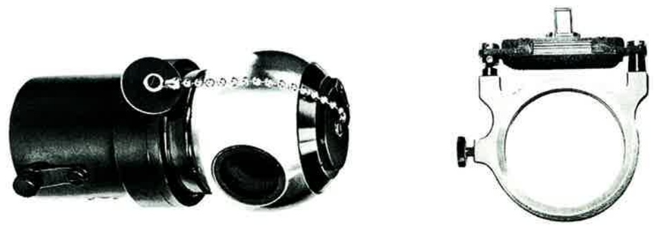
Figure 3-10. An optical square. It contains a pentaprism. Mounted on an alignment telescope, it will establish a plane perpendicular to the line of sight of the alignment telescope. The illustration at right shows a ring with a clamp and tangent screw (the index level) to control the slope of the right-angle line of sight.
