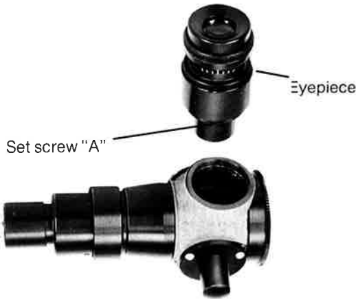
Figure A-5. Installation of Combination Auto-Collimation, Projection, Right-Angle Eyepiece
