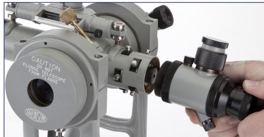
*8440 AlignCam eyepiece removal.*
